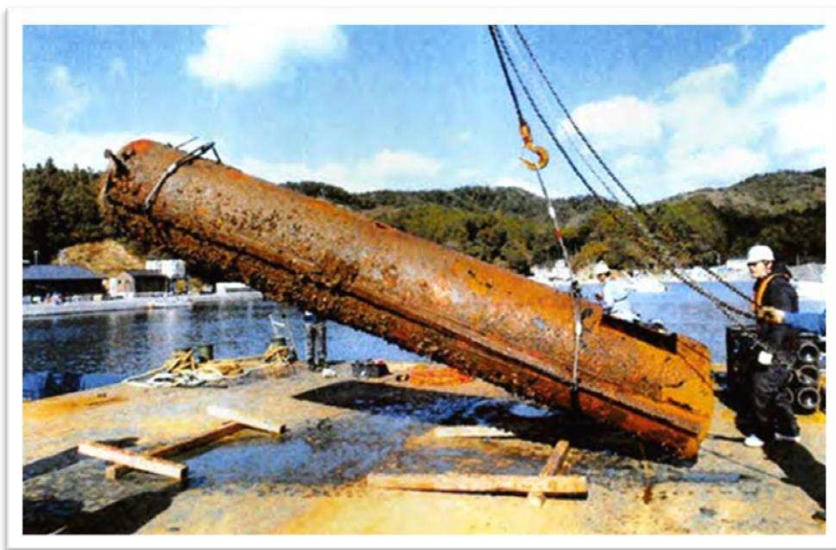
Photo n° 5: Pile n° 13 recovery (take from the document)
