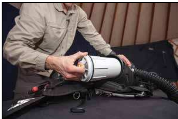
Figure 3. Cartridge containing carbon-dioxide absorbent material. Photo courtesy Jill Heinerth.
