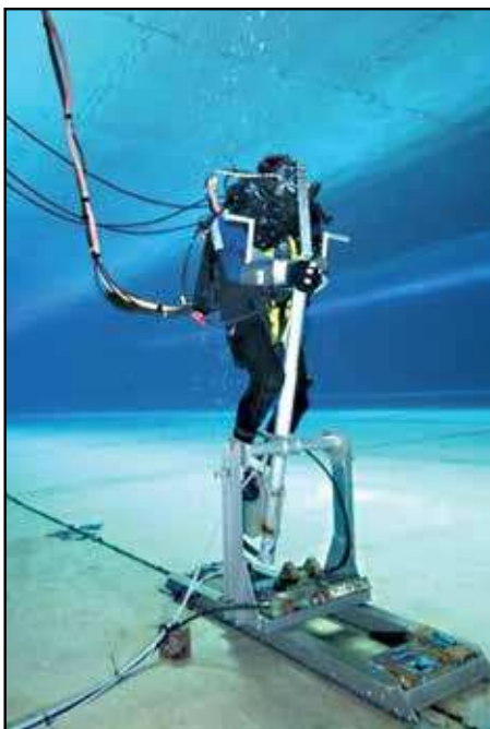
Figure 2. Controlled manned testing in a dive tank using a cycle ergometer.
