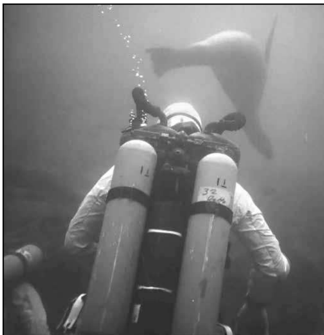
Figure 5. Back view of the U.S. Navy MK VI rebreather and a visitor to SEALAB II. U.S. Navy photo.
