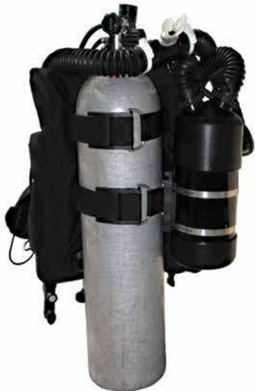
Figure 29. The KISS GEM semiclosed-circuit rebreather incorporating a standard aluminum 80 cu ft cylinder. Photo by Mike Young.
