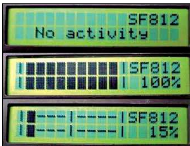
Figure 12. Photograph of the diver's display during different phases of a dive. The "SF812" refers to the absorbent used when the photo was taken.
