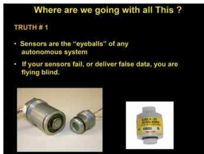
Figure 29. Typical sensors used in rebreathers: CO 2 sensors (left) and oxygen sensors (right). Do you trust their readings? How do you know?
