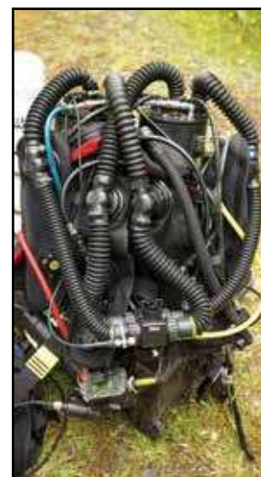
Figure 5. For deep dives in the Pearse Resurgence, Craig Challen uses a Twin Megalodon rebreather, with the two loops accessible by a custom-made dual bailout valve. This allows the diver to change from one loop to another with the flick of a switch. Photo by Richard Harris.
