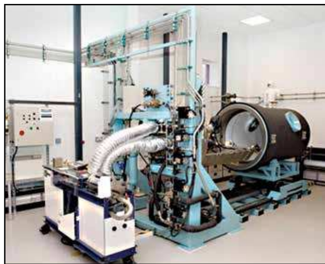
Figure 1. Unmanned test chamber and breathing simulator.
