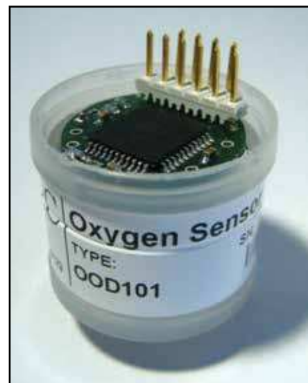
Figure 5. Prototype of our "smart" galvanic \text{O}_2 sensor.
