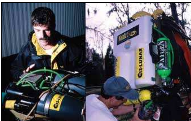
Figure 21. Final kitting up with the dual backmounted rebreather, January 1999. The small green tank is offboard oxygen; the small yellow tank is drysuit inflation argon supply. A second oxygen tank was placed inside the shell between the two CO 2 canisters.
